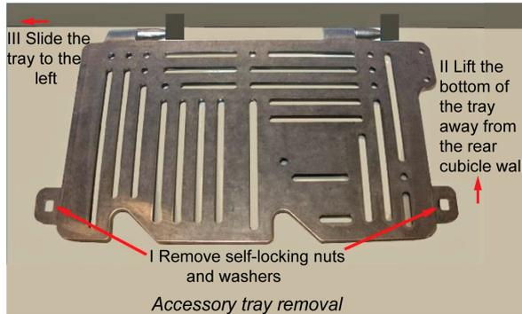
To install the upper tray, locate the accessory tray hinges to the left of the brackets in the top corner of the cubicle. Use the corner as a guide and slide the tray to your right. The self-locating hinges guide the tray into the brackets. Continue to slide the tray until the hinges are completely inside the brackets. Rotate the tray into the lock-down position and fasten the nuts.
